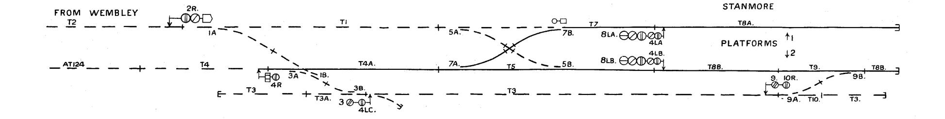
Trains arrive from Wembley at Stanmore at either platform 1 or 2 and can return to Wembley on the up line by AT 124 or can be shunted back from the shunt limit which is situated at about T4. 4R signals trains back into the platforms; 4LA, LB signal trains out of the platforms to shunt only, and 8LA, LB signal trains out of the platforms to Wembley.
